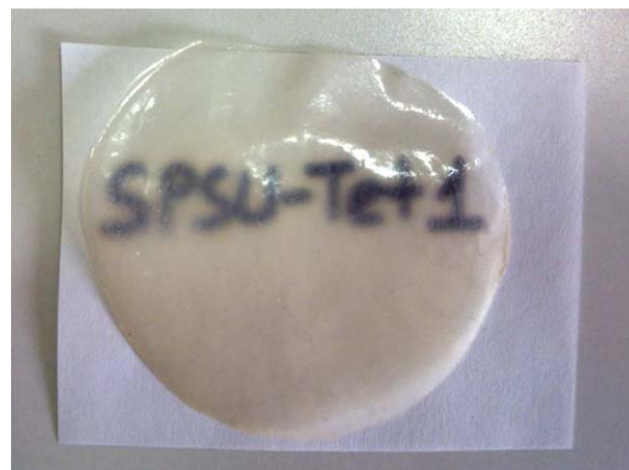
Figure 3. A picture of homogeneous and semitransparent SPSU–PMTet1 membrane. [Color figure can be viewed in the online issue, which is available at wileyonlinelibrary.com .]
